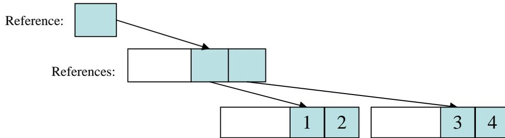
The likely size is  $3 * \text{sizeof}(\text{reference}) + 3 * \text{sizeof}(\text{heap\_overhead}) + 4 * \text{sizeof}(\text{double})$ . Assuming a reference to be one word and the heap overhead to be two words, we get a likely size of 17 words to compare to C++’s 8 words. This memory overhead comes with a run-time overhead from allocation and indirect access to elements. That indirect access to memory typically causes problems with cache utilization and limits ROMability.
