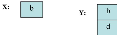
Only when we add virtual functions (C++'s variant of run-time dispatch supplying run-time polymorphism), do we need to add supporting data structures, and those are just tables of functions:
