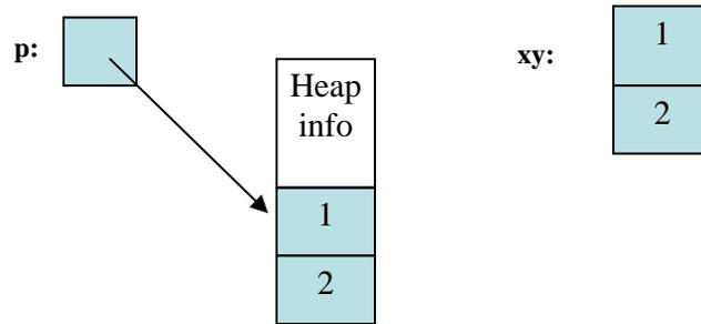
A **Point** is simply the concatenation of its data members, so the size of the **Point xy** is simply two times the size of an **int**. Only if we explicitly allocate a **Point** on the free store (the heap), as done for the **Point** pointed to by **p**, do we incur memory overhead (and allocation overhead). Similarly, basic inheritance simply involves the concatenation of members of the base and derived classes:
