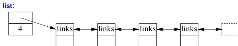
We use a `list` for sequences where we want to insert and delete elements without moving other elements. Insertion and deletion of phone book entries could be common, so a `list` could be appropriate for representing a simple phone book. For example:
