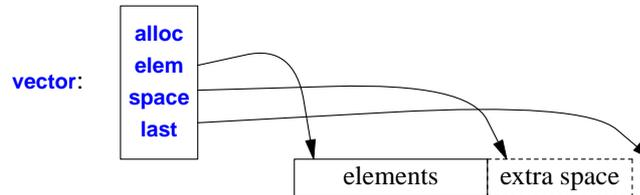
In addition, it holds an allocator (here, **alloc**), from which the **vector** can acquire memory for its elements. The default allocator uses **new** and **delete** to acquire and release memory (§12.7). Using a slightly advanced implementation technique, we can avoid storing any data for simple allocators in a **vector** object.
