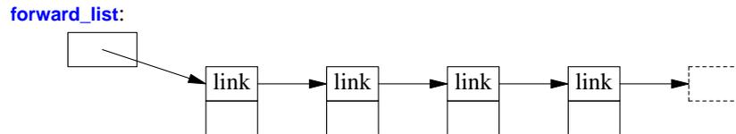
A `forward_list` differs from a (doubly-linked) `list` by only allowing forward iteration. The point of that is to save space. There is no need to keep a predecessor pointer in each link and the size of an empty `forward_list` is just one pointer. A `forward_list` doesn't even keep its number of elements. If you need the number of elements, count. If you can't afford to count, you probably shouldn't use a `forward_list`.
